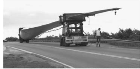
Figure 4-16. Specialized wheeled fixtures are required for transporting very long wind turbine blades. The blade shown here is 61.5 m long. (Courtesy of LM Glasfiber)
