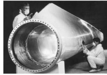
Figure 2.44. Rotor blade connection to the hub in the Vestas V-90 rotor blade
